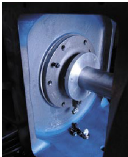
FIGURE 5-3 LOOSENING & REMOVING SEAL HOUSING & TOOL
