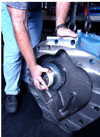
FIGURE 5-18 INSTALLING PLASTIC PROTECTIVE SLEEVE TOOL
