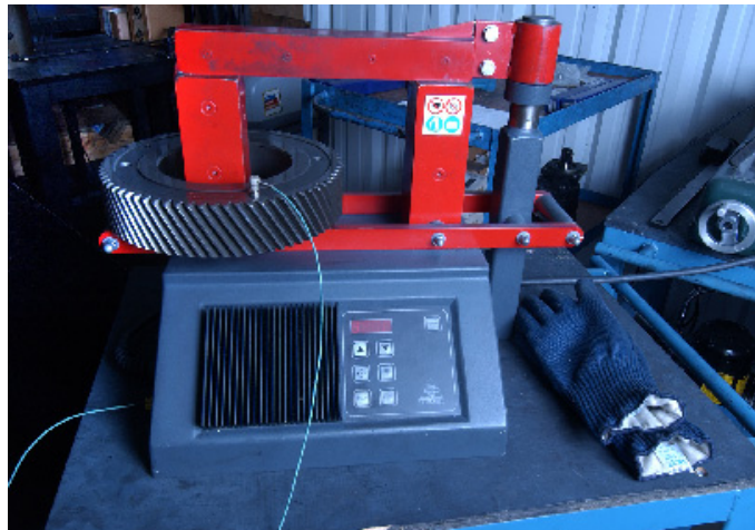
FIGURE 5-23 HEATING NEW GEAR
