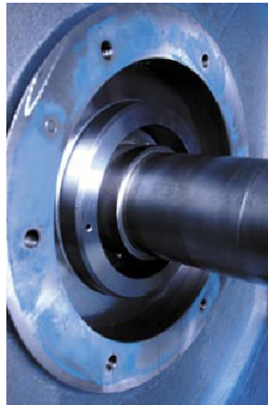
FIGURE 5-4 ROTATING HALF OF SEAL REMOVED
