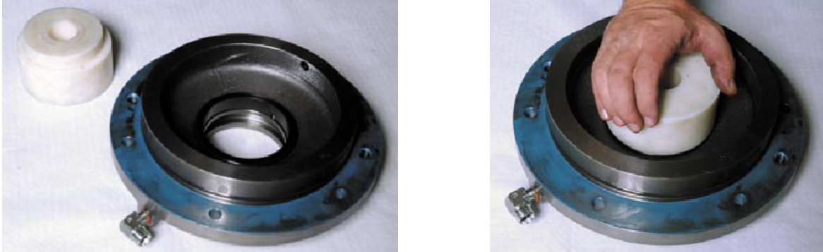
FIGURE 5-6 INSTALLING STATIONARY HALF OF SEAL
