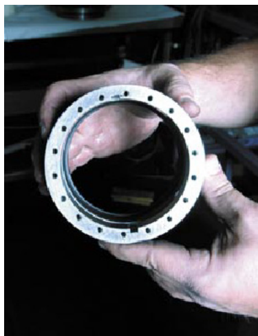
FIGURE 5-5 REAR VIEW ROTATING HALF OF SEAL
