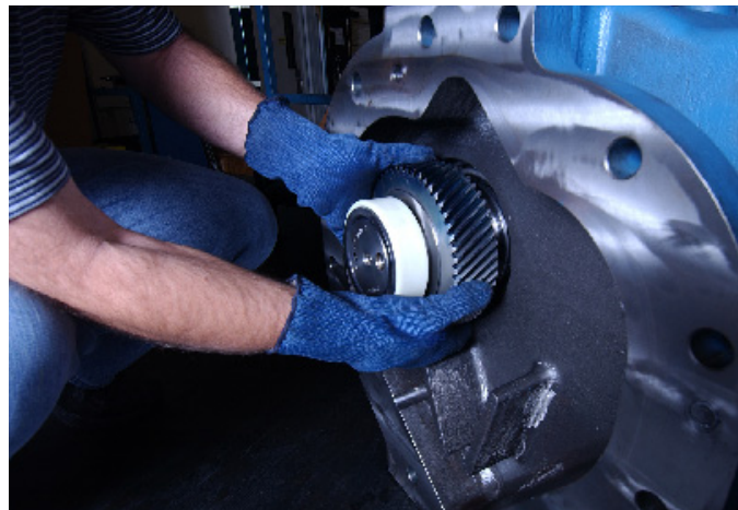
FIGURE 5-24 INSTALLING NEW GEAR
