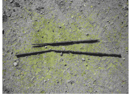
anode's after being removed from vessel.
